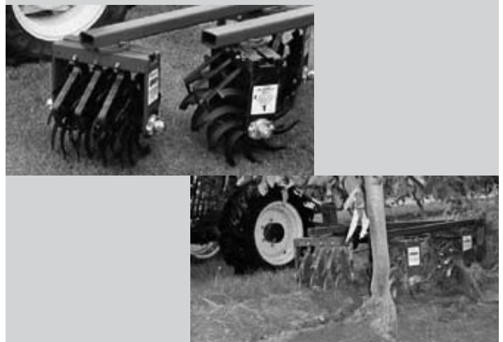
Wonder Weeder rotating tines attach to a hydraulic telescoping arm, increasing accuracy in orchard weed tilling. Photo by Wonder Weeder
