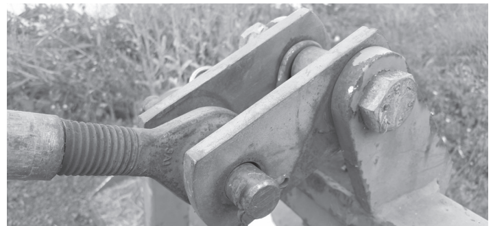
Easy to install, a floating attachment relieves the impact of an implement travelling over uneven ground or rocky fields.
