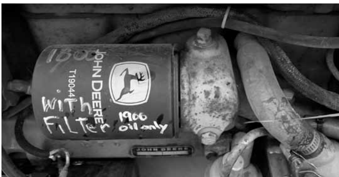
Figure 1: You can write the date and service hours right on your engine.
